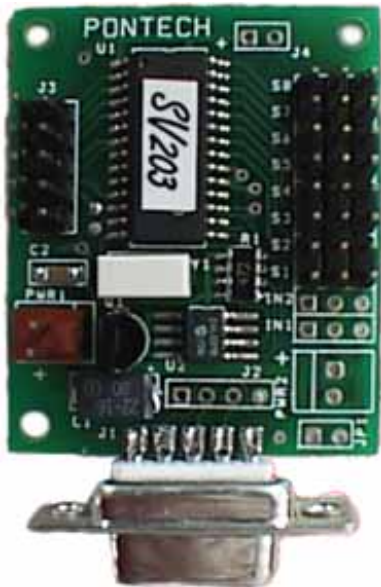
Figure 2. The Servo Controller Board. The pins to the right control servo motors, while the pins at left measure analog voltages.
