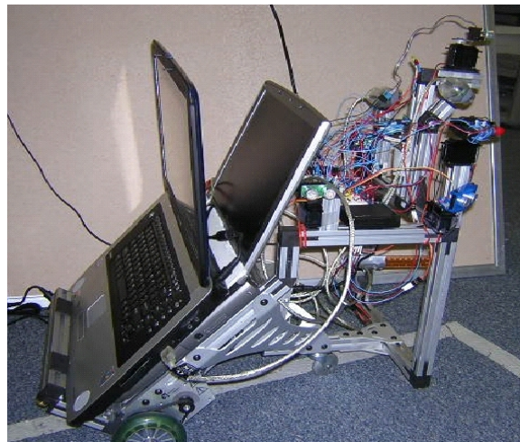
Figure 1. Our robot used an array of servo-mounted sonar sensors and a laser-pointer-based range finder. The chassis is an Evolution ER1; two laptops provide its computational engine. Without the laptops the platform totals $600.
