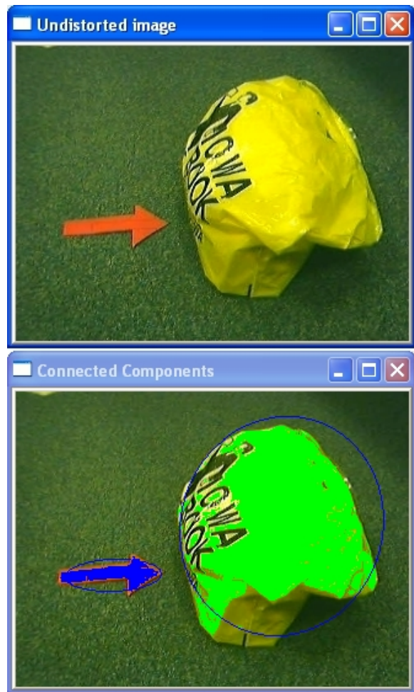
Figure 4: A raw image and the results of segmentation, connected components, and shape processing: best-fit ellipses surround both the arrow and the yellow bag.
