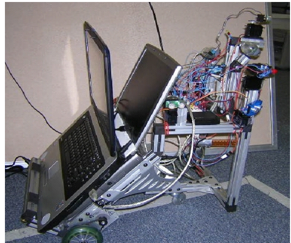
Figure 1: The laptop-controlled scavenging robot built atop an Evolution ER1. The sensor suite points toward the typical direction of travel, and onlookers can follow the robot’s reasoning by watching the screens from behind. Both custom and commercial interface circuits mediate between the two sides.
