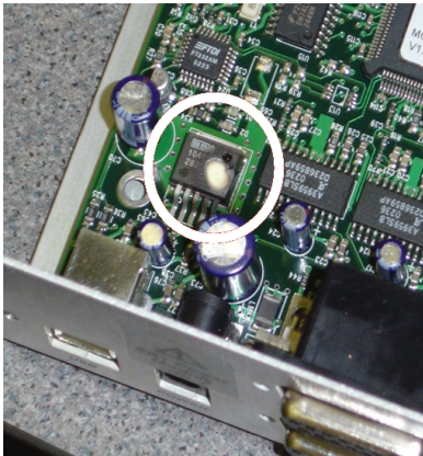
Figure 7: One of the power regulators within Evolution Robotics' early Robot Control Modules looking a bit worse for wear...
