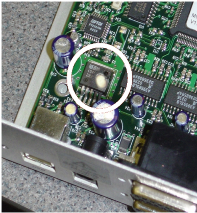
Figure 7: One of the power regulators within Evolution Robotics' early Robot Control Modules looking a bit worse for wear...
