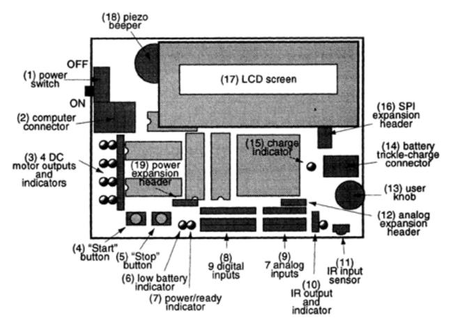
The figure above shows a labelled view of the base Handy Board's ports, connectors, inputs, and outputs. The expansion board is not shown, but is shown in the following photo. Below, each of these parts is briefly described.
