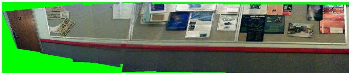
Figure 8: Rendering of the "hallway" map. Though only a single plane, this map fuses the 10 images from the red portion of the path in figure 1. To the left appear the visual repercussions of a rotation not modeled by the robot's odometry. Such artefacts argue for adjusting the odometric poses based on future data, i.e., SLAM.
