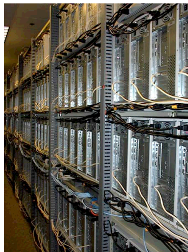
Koza's 1000 node Beowulf used for genetic programming
