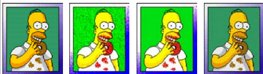
original 8 bits/pixel/channel random ordered error-diffusion 1 bit/pixel/channel
