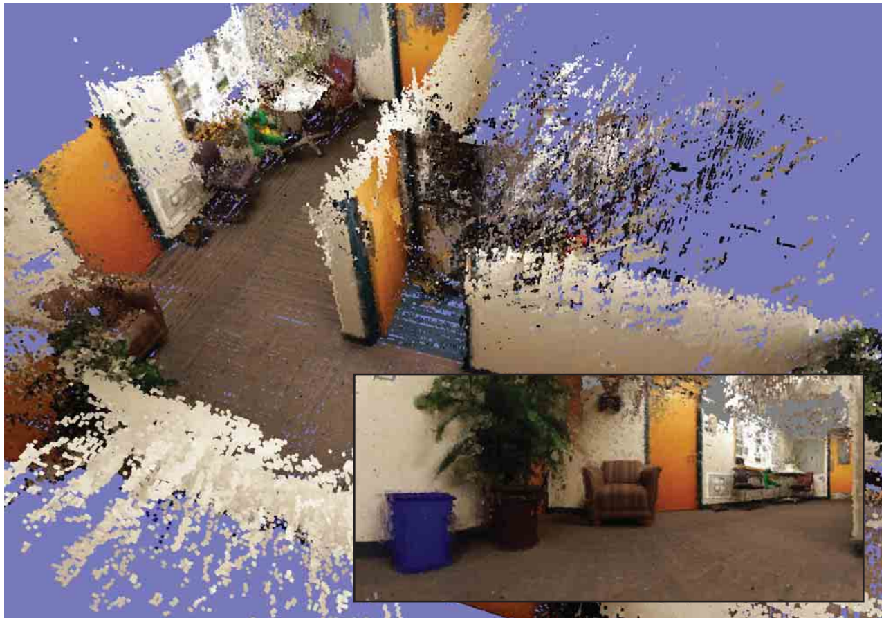
Figure 2. Overview and interior views of a 3D map generated by Seegrid Corp. programs using only stereoscopic camera views from a robotic vehicle's trip down the center of an L-shaped hallway.
