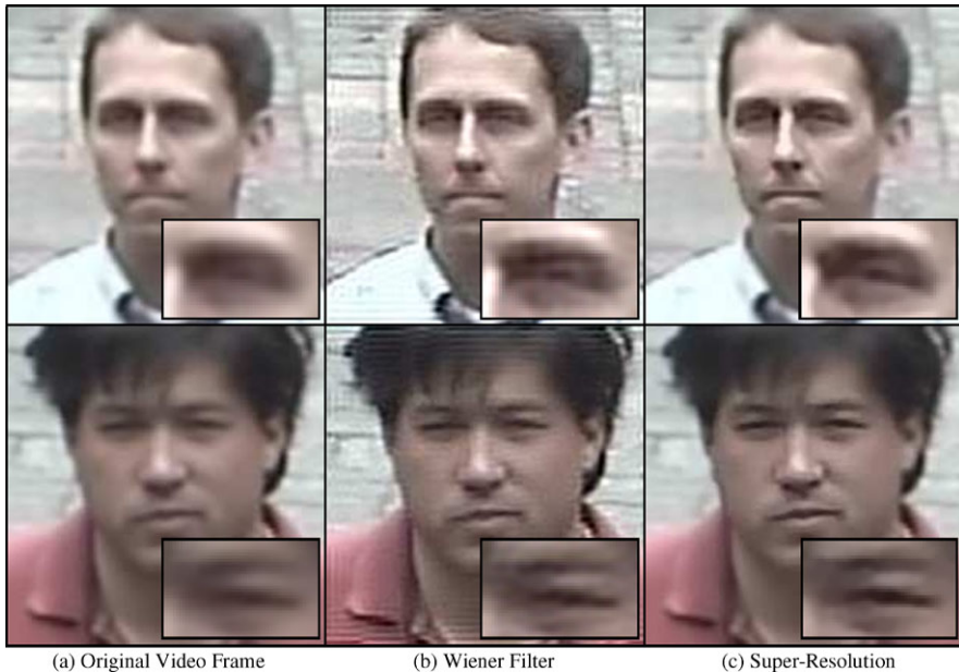
Fig. 14.12 Example original video frames, Wiener filter results, and super-resolution results with enlarged views of the left eye. In the Wiener filter results, artifacts in the face region are primarily due to enhancement of interlacing artifacts. Some ringing due to circular convolution is present, but only near the image edges. The increased resolution and clarity in the super-resolution results is clearly visible (© 2009 IEEE, used with permission [55])
