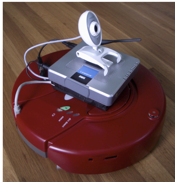
Figure 2 Autonomous Linux Roomba utilizing a WRTSL54GS, USB webcam, flash drive, and serial port.
