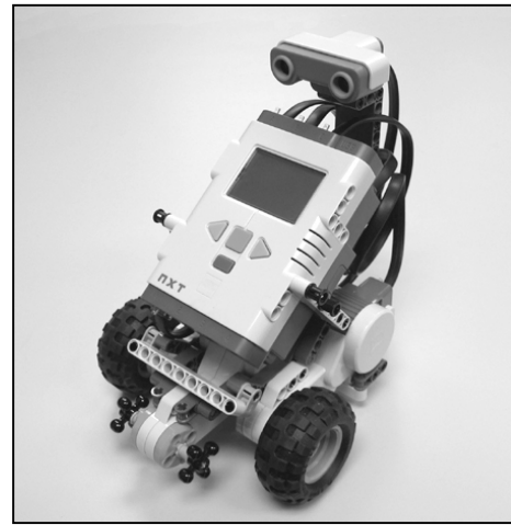
Figure 2: NXT with Sonar Sensor
