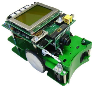
Figure 1: SoccerBot mobile robot and EyeBot controller
