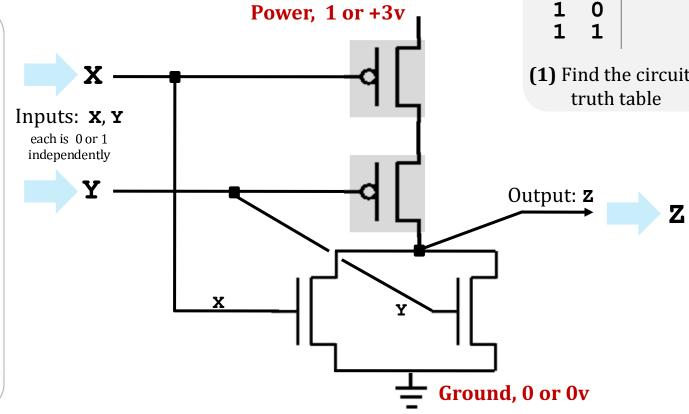
(3) Extra! How could you alter the transistor-level design to make an AND?
