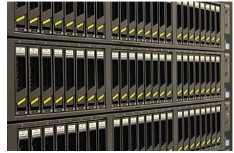
Storage servers with 24 hard disk drives each and built-in hardware RAID controllers supporting various RAID levels
