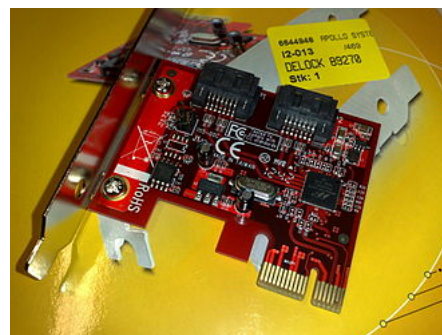
A SATA 3.0 controller that provides RAID functionality through proprietary firmware and drivers
