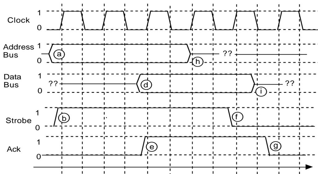
**Figure 293: Handshaking sequence for a memory read**
