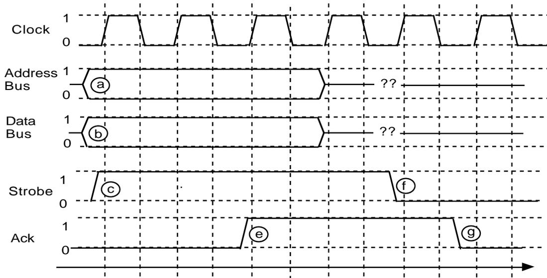
**Figure 294: Handshaking sequence for a memory write**
